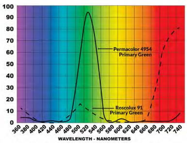
Another feature of dichroic filters is that they produce higher, more precise light transmission. When compared side-by-side, Permacolor dichroic filters provide higher transmission and colour purity than their equivalent hues in Roscolux, Supergel, GamColor or e-Colour+.
