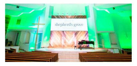
The cross, which is prominently featured on the altar, was falling flat on-camera and needed a bit of a boost. The team at PCE originally tried to front light it, but they moved away from that technique because of the difficult hanging points in the space and the fact that the wall wash behind the cross was too overpowering. Instead, they decided to back light the cross in a contrasting/complementary color to the back wall's lighting scheme.
