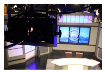
Thanks to the unique design of the Braq Cubes, two units can be ganged together on one yoke for extra output.
