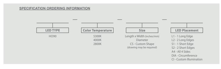
**HO90 - 5300K - 12 in x 12 in - A4** specifies a 12 in square LitePad with a color temperature of 5300K and LEDs on all sides. **HO90 - 2800K - 200 mm - DIA inside** specifies a 200 mm round LitePad with a color temperature of 2800K and LEDs on the inside circumference.
