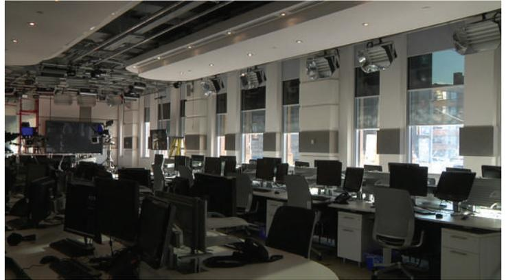
Manual or motorized controlled RoscoShades allow the user to lower a variety of different densities of Rosco Neutral Density Filter, Scrim and Color Correction Filters in front of the windows. By varying the combination of materials, the Lighting Director can closely match the exterior exposure to their interior lighting.
